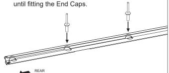
Slide the end cap into the correct track end. Make sure that the hole on the end cap lines up with the hole on the track before riveting in place.
