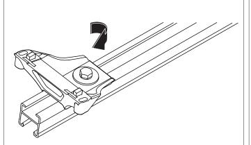
Check that the channel nut is fully located across the bar.
