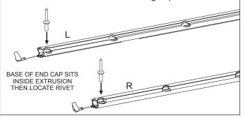
Using either a pneumatic or concertina type rivet gun, rivet track and end caps into place, making sure all rivets are seated firmly onto the base of the track.
