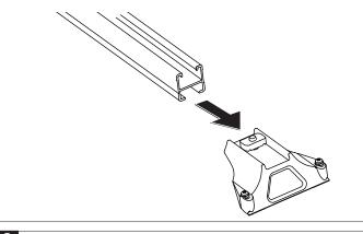
Finger tighten the leg attachment bolt so that the channel nut turns to locate across the cross bar. The legs will require adjustment later.
