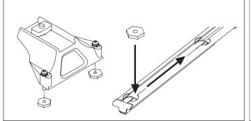
Slide the cross bar onto the leg and locate with the M10 channel nut. Leave untensioned at this stage.
