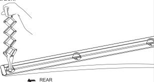
The original roof trim will have to be measured and cut once the tracks are riveted in place. Make sure the front end of the trim sits correctly under the windscreen rubber before measuring and cutting. When cut (using a Fine Tooth Hacksaw) the roof trim must butt up against the Track End Cap.
